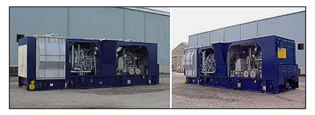
Fuel:Liquid/Gas FiredRating:ISO rated @ 39.5MW: (Gas fired )Voltage:11.5KvPhase:3Frequency:50 Hz-pf :0.8Units can also be upgraded to 41 MW
